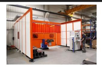
A form of room ventilation system helps prevent this. At the end of the cabin, the ventilation system continuously extracts the contaminated air out of the cabin. A central filter system connected to the cabin extracts the hazardous substances and directs the clean air back into the hall. Because this results in air constantly flowing into the cabin from the hall, it prevents the welding fumes from escaping.
