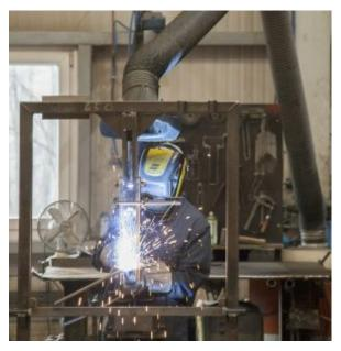
In practical applications that is not always a given, which means that avoidable mistakes can often be observed: The extraction hood rests, for example, above the welder's head towards the welding point and is not tracked at any point. Thus, he first inhales the welding fumes before it they are captured by the extraction plant. Or the extraction arm is positioned too far away from the source of the welding fumes and the extraction effect becomes ineffective.
