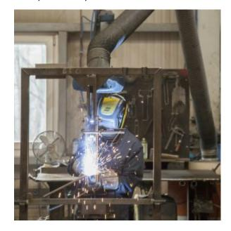
In practical applications that is not always a given, which means that avoidable mistakes can often be observed: The extraction hood rests, for example, above the welder's head towards the welding point and is not tracked at any point. Thus, he first inhales the welding fumes before it they are captured by the extraction plant. Or the extraction arm is positioned too far away from the source of the welding fumes and the extraction effect becomes ineffective.
