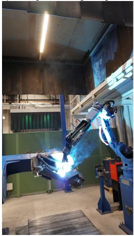
technology. Two extraction bonnets of the appropriate size, adapted to the respective work areas, also ensure that the welding fumes do not spread into the ambient air thanks to the lamellas on the side edges. In the robot grinding cell, too, the extraction takes place directly above the point of origin.
