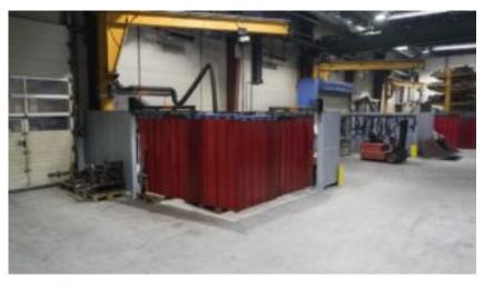
made air pollution control concept for the welding shop along the special requirements. Using 3D visualisation, the extraction specialist made the planning comprehensible at all times. In order to create a positive overall working environment, the end result was a mix of different protective welding equipment. The focus was not only on the welders' working area, but on the entire indoor air quality.
