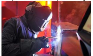
composition. The inert gas carbon dioxide becomes e.g. carbon monoxide during MAGC welding. Furthermore, the arc also has an effect on the creation of hazardous substances. MAG welding is an arc welding process: An endless wire electrode melts underneath an inert gas cover which protects against the atmosphere.
