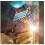
Particulate substances have to be considered during risk assessment. Toxic substances such as manganese oxide, which is created when MAGM-welding of chrome-nickel steel with solid wire, irritate the respiratory tract in high concentrations and may damage the nervous system. Nickel oxide can cause cancer when used in the same process - just as much when using chrome VI compounds for MAGM-welding of chrome-nickel steel with cored wire electrode.
