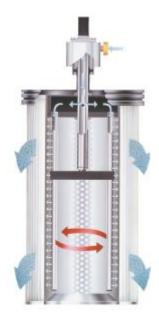
Which filter technology is the right one for the respective requirements of the metal processing company depends on the purpose and duration of use. When it comes to extraction in heavily fuming processes, there is no alternative to cleanable filter media. If fumes emission is comparatively low and the unit is only used for a few hours a day, the cheaper filter unit with storage filters may be the right choice.
