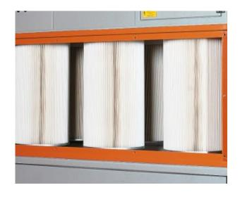
If you weld with high intensity and generate large quantities of welding fumes, then you require a larger filter area than sporadic welders. The larger the filter surface is, the greater the filters so called dust storage capacity is and therefore its service life before the next filter change.
