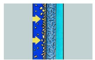
In contrast to this is the filter technology of the cleanable filters: Welders opt for this to avoid regular changes. It is true that costs for the initial purchase of the extraction unit are usually higher than with disposable filter units, but the investment quickly pays for itself where fumes are considerable and/or a lengthy operating period is involved.
