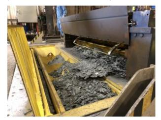
Cleaning may last several hours, if not days. It is a dirty and hazardous operation in which the employees are exposed to dust which is hazardous to health. During this time, the machine is at a standstill which, in turn, leads to considerable downtimes. Given the high cost of purchasing new cutting machines, companies try to keep downtimes as low as possible in practice.
