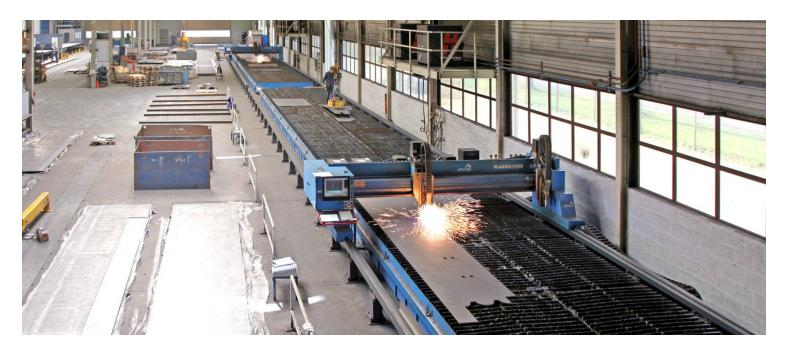
Wherever welding takes place, an extraction table is normally not far off. It is not just used as a material support, but also ensures the safety of the employees from the large fine dust volumes when operating the cutting plant - seven facts on what makes an effective extraction table.
