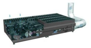
surface of the table into the inside of the table. This is regulated for certain cutting tasks in the norm DIN EN ISO 17916. Furthermore, it is essential that the cutting beam can stream at first as easily as possible into the table and then only rise back up after a deflection. Slag and a large part of the sparks are already separated into the slag tanks. Then the extraction slots in the upper area of the extraction table capture the smoke which is rising again due to its thermal
