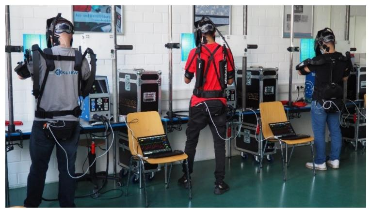
Exoskeletons are already being used in numerous industries such as logistics or the automotive industry and even in healthcare. They enable employees to maintain an ergonomic posture and minimise negative effects on the musculoskeletal system due to one-sided physical activities. They support the movements of the wearer. Depending on their needs, they can also amplify movements with the help of small drives on the joints of the exoskeletons.
